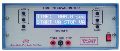
Type 1425 series Micro controller based Digital Time Interval Meters are used for the measurement of time interval from  $100\mu$  sec. to 9999 secs. (2 hrs. 45 mins.). This is ideally suited for measuring switching time of relays, trip time & on time of circuit breakers, fusing time of fuse elements, travel time of switches and contactors etc. Type 1425 series can also be used as an accurate Stop Watch by stop watch switches.
