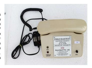
This is designed to replace Conventional Magneto Telephone with hand cranking, generator thus named as Electronic Magneto Telephone.
