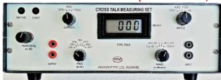
As the measuring range starts from zero dB the instrument can conveniently be used for measuring transmission losses in cable, thus working as a Transmission Measuring Set.
