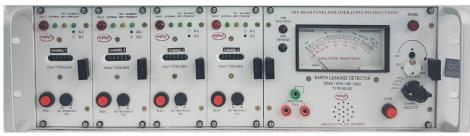
set value. Each such fault is recorded on a 6-digit counter. Fault detection can be set in between 2K-1MΩ. The audio alarm is common for all Channels while the visual indication is separate for each channel.
