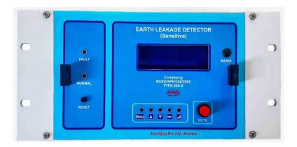
ELD (Sensitive) continuously monitors the condition of the cable and an alarm is actuated along with a visual indication when the leakage value drops below the pre-set value. This value can be set between 50 K to 1M Ohms. Relay contacts are available for connecting to a data logger for automatic recording of the faults occurred.
